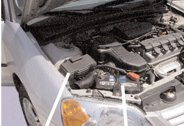
Under-Hood Fuse Box
